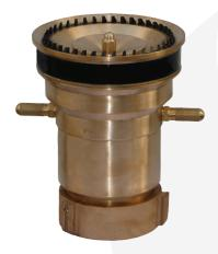
The debris trapped in the nozzle may effect the nozzle performance. To remove trapped debris, the water flow must be stopped and thereafter carefully unscrew and remove the nozzle deflector. Clean the nozzle and reassemble.
