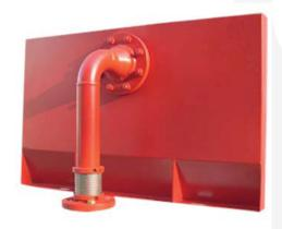
The foam is produced by introducing air into the foam solution stream. The inlet of foam maker is designed to create venturi jet which draws air into the foam solution stream. The air is drawn into the foam solution through holes located on the foam maker covered with stainless steel screen to exclude nesting birds and insects.
